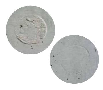
Due to 220 g /m<sup>2</sup> phenolic resin coating and waterproof film on the reverse side hardly any marks on the concrete!
